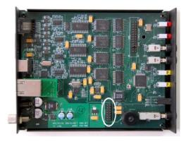
Remove the top cover of the LD-350 by removing the four cover screws. Locate the relay connector by the side of the unit behind the power switch.
