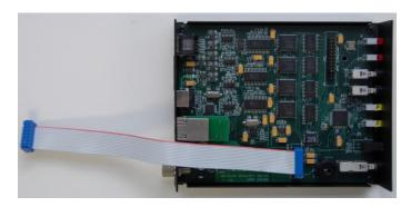
Plug the ribbon cable into the relay connector as shown. The relay connector pin 1 must plug into the ribbon cable connector holes closest to the red stripe. The other end of the ribbon cable connector at the rear of the LD-350 should be facing upwards as shown.
