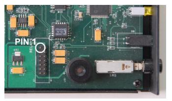
Locate pin 1 of the relay connector. Pin 1 is towards the center of the LD-350. The female ribbon cable connector and the LD-350 have 14 holes/pins (2x7). It is important that pin 1 is inserted into the connector holes closest to the ribbon cable's red stripe.
